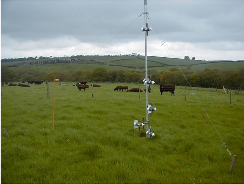
IHF Mass Balance technique with passive NH 3 samplers
