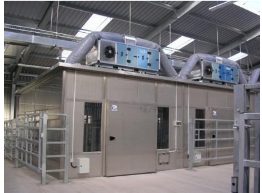
Animal respiration chamber – CO 2 and CH 4 emissions
